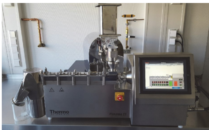
Fig. 2: Pharma 11 extruder with granulation kit
